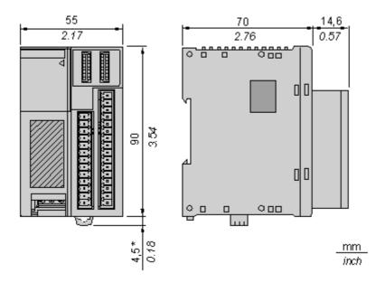
NOTE: \* 8.5 mm (0.33 in) when the clamp is pulled out.
