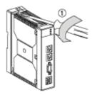
Step 2: Pivot the module forwards and disengage the pins from the holes located in the bottom of the support.
