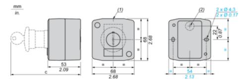
(1) 2 knock-outs for Pg 13.5 cable gland, maximum capacity 12 mm/0.47 in. (2) Knock-out for cable entry, maximum capacity 14 mm/0.55 in.
