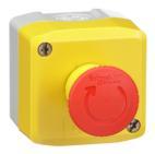
Control station, Harmony, plastic, yellow, 1 red mushroom head push button 40mm, emergency stop turn to release 1NO + 1NC, unmarked, UL CSA certified
