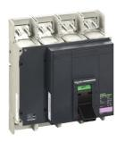
Basic switch disconnector, ComPact NS1250NA, withdrawable, manually operated, 1250A, 690VAC 50/60Hz, 4P
