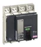
Circuit breaker, ComPact NS1000N, 50kA/415VAC, Micrologic 6.0 trip unit, 1000A, fixed, 4 poles 4d
