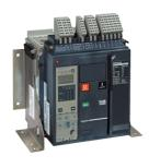
Circuit breaker frame, MasterPact NT16H1, 1600A, 42kA/440VAC 50/60Hz (Icu), 3 poles, fixed, without control unit
