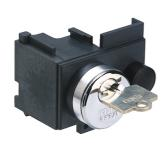
Circuit breaker locking, MasterPact NT fixed/drawout, OFF position locking, Ronis keylock, 2 locks, 1 key
