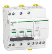
Residual current breaker with overcurrent protection (RCBO), Acti9 iCV40N, 3P+N, 20A, C curve, 6000A, AC type, 30mA
