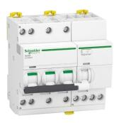
Residual current breaker with overcurrent protection (RCBO), Acti9 iCV40N, 3P+N, 32A, C curve, 6000A, A-SI type, 30mA
