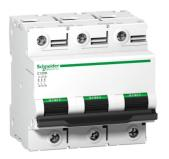
Miniature circuit breaker (MCB), Acti9 C120N, 3P, 63A, B curve, 10000A (IEC/EN 60898-1), 10kA (IEC/EN 60947-2)
