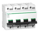
Miniature circuit breaker (MCB), Acti9 C120N, 4P, 63A, B curve, 10000A (IEC/EN 60898-1), 10kA (IEC/EN 60947-2)
