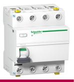
Residual current circuit breaker (RCCB), Acti9 iID, 4P, 100A, A-SI type, 300mA, selective, double terminal
