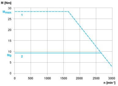
Servo Motor with LXM28AU20 ••• Servo Drive
