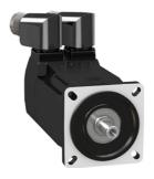
servo motor BMH, Lexium 32, 1.2Nm, 8000rpm, keyed shaft, without brake, IP54, 16bit encoder
