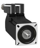
servo motor BMH, Lexium 32, 1.2Nm, 8000rpm, keyed shaft, without brake, IP65, IP67, 128 multiturn encoder
