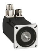
servo motor BMH, Lexium 32, 1.4Nm, 8000rpm, untapped shaft, without brake, IP54, 16 multiturn encoder, straight
