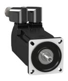
servo motor BMH, Lexium 32, 2.5Nm, 8000rpm, keyed shaft, without brake, IP54, 128bit encoder, 3 phases
