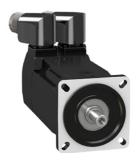
servo motor BMH, Lexium 32, 3.4Nm, 8000rpm, keyed shaft, without brake, IP54, 128 multiturn encoder, 3 phases
