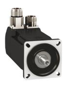
servo motor BMH, Lexium 32, 3.4Nm, 8000rpm, keyed shaft, with brake, IP54, 128 multiturn encoder, straight, 3 phases
