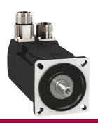
servo motor BMH, Lexium 32, 3.4Nm, 8000rpm, untapped shaft, with brake, IP65, IP67, 16bit encoder, straight
