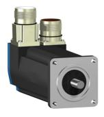
servo motor BSH, Lexium 05, 0.9N.m, 4000rpm, 55mm, untapped shaft, Sincos multi turn, without brake, IP50, straight
