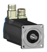
servo motor BSH, Lexium 05, 1.4N.m, 3000rpm, 70mm, keyed shaft, Sincos single turn, without brake, IP50, straight
