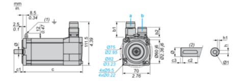
a: Power supply for servo motor brakeb: Power supply for servo motor encoder
