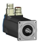
servo motor BSH, Lexium 05, 1.1N.m, 3000rpm, 70mm, keyed shaft, Sincos multi turn, without brake, IP50
