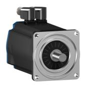
servo motor BSH, Lexium 05, 7.8N.m, 2500rpm, 100mm, untapped shaft, Sincos multi turn, with brake, IP65
