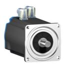
AC servo motor BSH, Lexium 05, 19.5N.m, 1500rpm, untapped shaft, without brake, IP50
