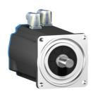
servo motor BSH, Lexium 32, 32.1N.m, 3000rpm, 140mm, untapped shaft, Sincos single turn, without brake, IP50
