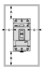
Toggle-type, rotary handle-type: identical clearance values.
