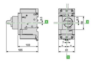
GV4L, GV4P, GV4LE, GV4PE, GV4PEM Panel Mounting with M4 Screws
