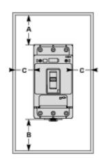
Toggle-type, rotary handle-type: identical clearance values. Safety Clearance (mm)
