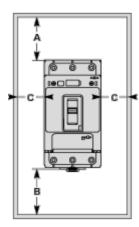
Toggle-type, rotary handle-type: identical clearance values
