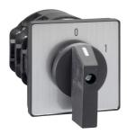
Cam changeover switch, Harmony K, front mounting, plastic, 4 poles, position 0, 60°, 150A, 88x88mm, marked 1/0/2
