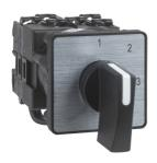
Cam changeover switch, Harmony K, multifixing, plastic, 4 poles, position 0, 45°, 20A, 45x45mm, metallic legend, marked 2/0/1, 35mm black handle
