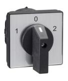
Complete cam switch, Harmony K1, K2, cam changeover switch, front mounting, plastic, 4 poles, position 0, 60degrees, 50A, 64x64mm, marked 1 0 2
