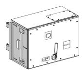
Plug-in tap off unit, Canalis KH, with switch disconnector for DIN fuse size 3, 630A, 3L+PEN, right cable exit, RAL9001
