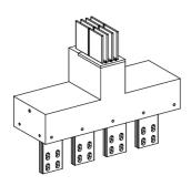
Straight feed unit, Canalis KRA, aluminium, 800A, 3L+N+PE, made to measure dimensions, flat connection pads, RAL7030
