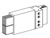
Adaptor, Canalis KRC, copper, 2000A, 3L, fixed length 600mm, interconnection with Canalis KTC 3L+PE
