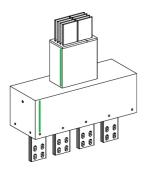
Straight feed unit, Canalis KRC, copper, 5000A, 3L+N+PE, made to measure, flat incoming and connection pads, RAL7030
