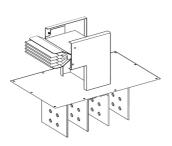
Flat elbow feed unit, Canalis KTA, aluminium, 1000A, 3L+N+PE, made to measure dimensions, neutral N3, white RAL9001
