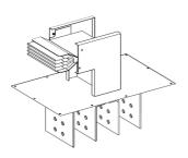
Flat elbow feed unit, Canalis KTA, aluminium, 1000A, 3L+N+PER, made to measure dimensions, neutral N3, white RAL9001
