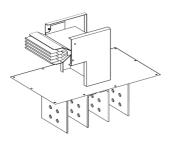
Flat elbow feed unit, Canalis KTA, aluminium, 1000A, 3L+N+PER, made to measure dimensions, neutral N4, white RAL9001
