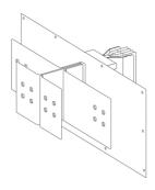
Bar feed unit, Canalis KTA, aluminium, 1000A, 3L+N+PER, flat outlets, made to measure dimensions, neutral N7, RAL9001
