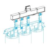
Feed unit for dry type transformers, Canalis KTA, aluminium, 1600A, 3L+N+PE, made to measure, neutral N3, white RAL9001
