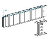
Straight transport length, Canalis KTA, aluminium, 2500A, 3L+N+PE, high Icw, made to measure length 2-2.5m, RAL9001
