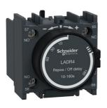
Time delay auxiliary contact block, TeSys Deca, 1NO+1NC, off delay 10-180s, front, screw clamp terminals
