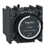
Time delay contact block,TeSys Deca,1NO+1NC,on-delay 1-30s,front,with 40±15ms switching time between NC opening and NO closing
