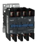
Contactor, TeSys Deca S207, 4P(4NO), AC-1, <=440V, 125A, 24V DC wide range coil, ring-lug terminals
