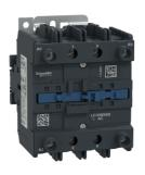
Contactor, TeSys Deca, 4P(2NO+2NC), AC-1, <=440V, 125A, 110V AC 50/60Hz coil, screw clamp terminal
