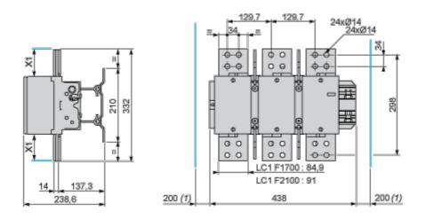
(1) Minimum distance required for coil removal.
