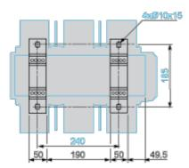
**NOTE:** X1 (mm) = Minimum electrical clearance according to operating voltage and breaking capacity.
